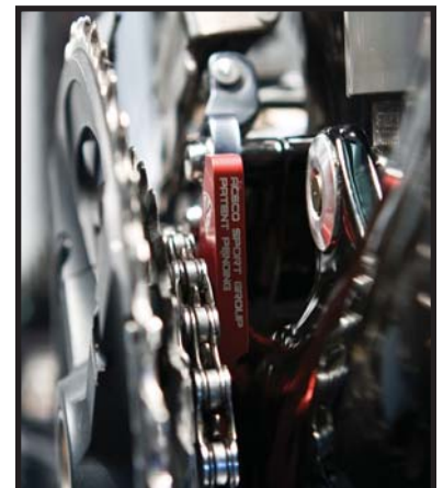
Fig 9 – Chain Clearance with K-Edge Dirt Triple Installed
