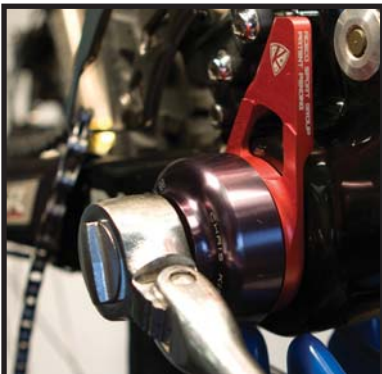
Fig 6 – Positioning and Tightening of BB Cup and K-Edge
