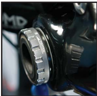
Fig 2 – BB with 2.5mm Spacer
