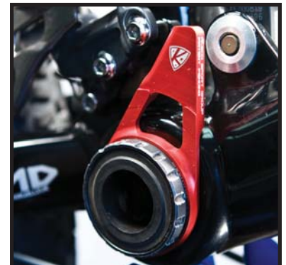
Fig 7 – Position of K-Edge with BB Cup Installed
